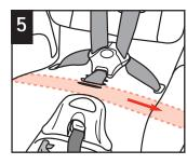
Pull other end of LATCH hook **under** pad in front of crotch strap to the opposite side. Do not place LATCH belt over child's legs.
